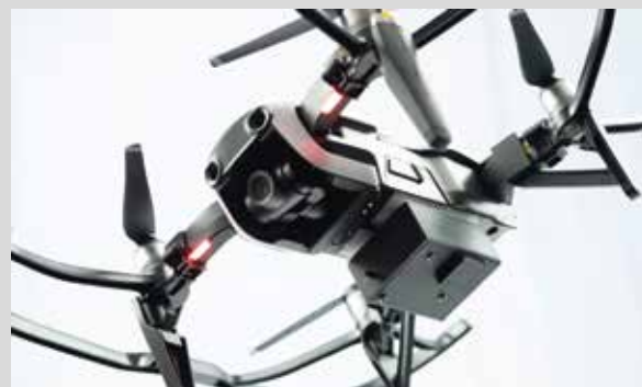
Remote pipework cutting operations (top) Lightweight embeddable module for aerial radiological investigation
