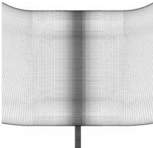
**FIGURE 5: Planar cross-section of the LES mesh at the injection inlet T-junction.**
