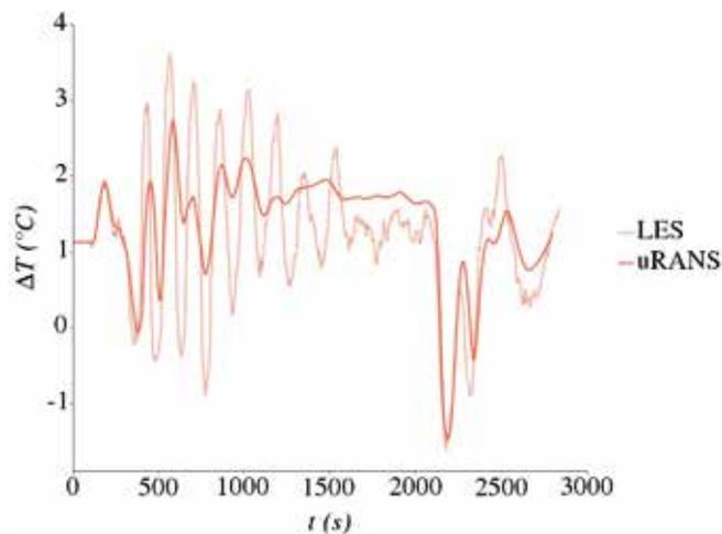
**FIGURE 7: Temporal evolution of  $\Delta T$ , where cold fluid was injected at a rate of 0.1 kg/s from  $t = 100$  s to  $t = 2100$  s.**
