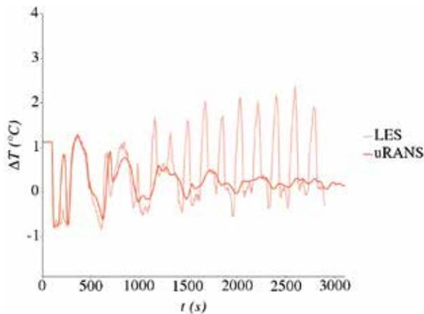
**FIGURE 9: Temporal evolution of  $\Delta T$ , where the heater was switched off at t = 100 s.**
