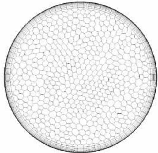
FIGURE 2: Circular cross-section of the RANS mesh in the stream direction.
