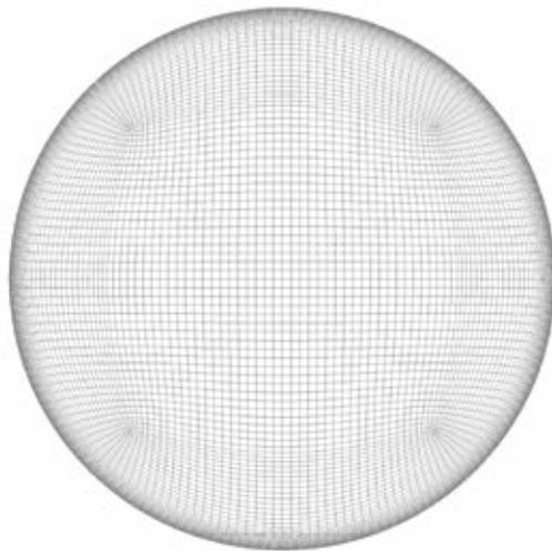
**FIGURE 4: Circular cross-section of the LES mesh in the stream direction.**
