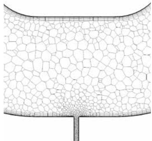
FIGURE 3: Planar cross-section of the RANS mesh at the injection inlet T-junction.
