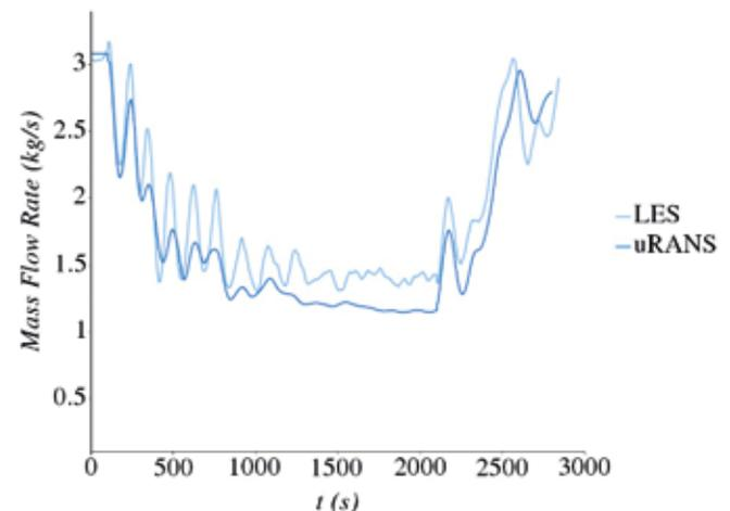
**FIGURE 6: Temporal evolution of mass flow rate, where cold fluid was injected at a rate of 0.1 kg/s from  $t = 100$  s to  $t = 2100$  s.**
