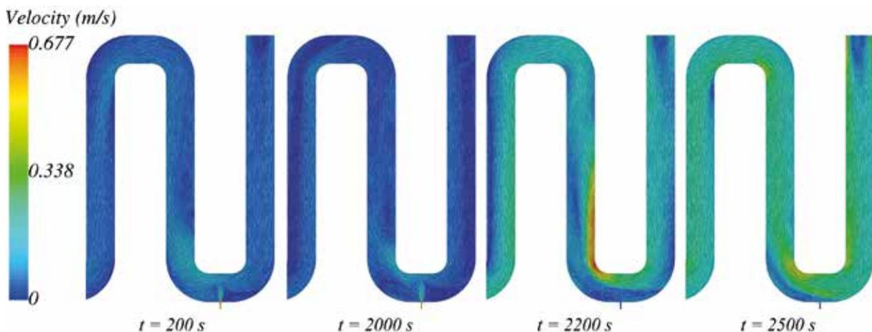
**FIGURE 11: Intermittent velocity contour plots of the loop seal, where cold fluid was injected at a rate of 0.1 kg/s from  $t = 100$  s to  $t = 2100$  s.**
