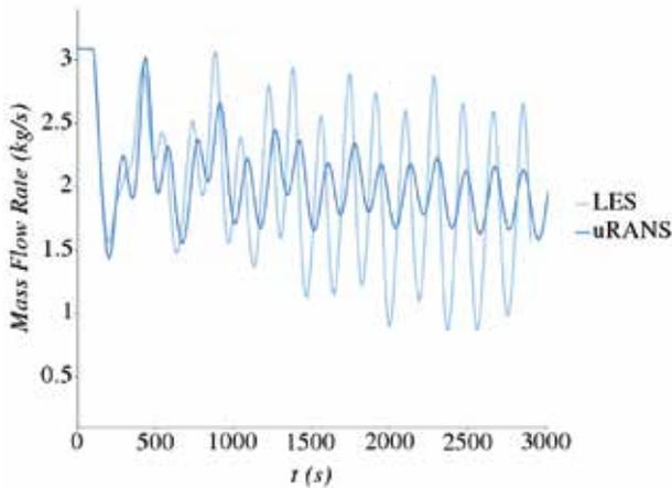
**FIGURE 8: Temporal evolution of mass flow rate, where the heater was switched off at t = 100 s.**
