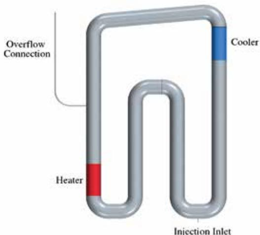
FIGURE 1: Image illustrating the geometry of the NC loop.
