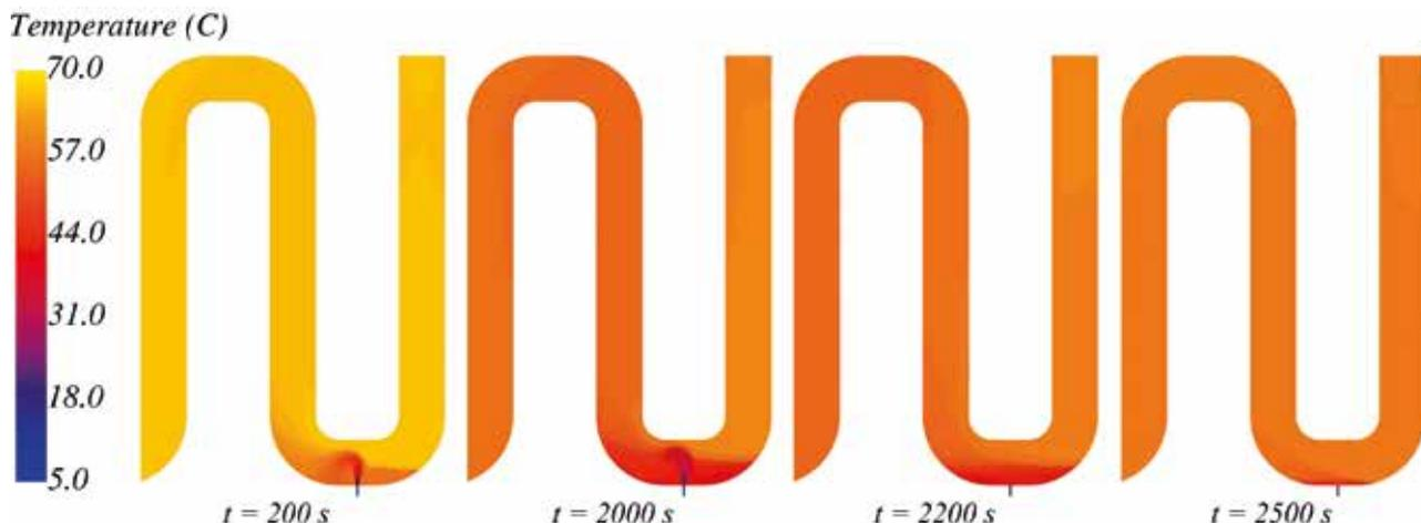
**FIGURE 10: Intermittent temperature contour plots of the loop seal, where cold fluid was injected at a rate of 0.1 kg/s from  $t = 100$  s to  $t = 2100$  s.**
