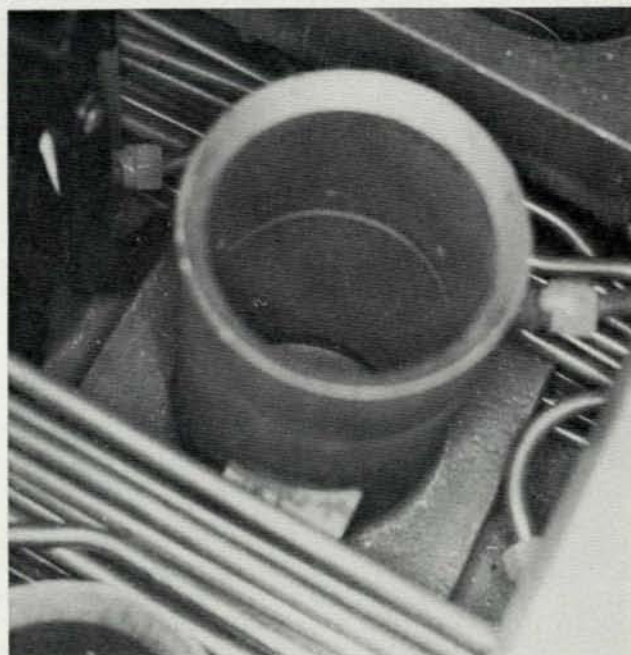
Fig 17 BCD tubes trapped under charge pot
